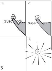
Unlock the settings by long pressing key "O" for 3 seconds.
