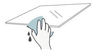
5. Carefully remove the glass from the oven door. The number of glass panes may vary depending on your model. Wipe clean with a soft, damp cloth and mild detergent.
