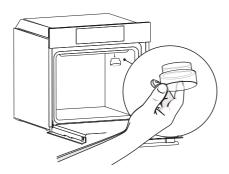
To remove your light bulb, undo the glass cover, unscrew the bulb and replace it with a new bulb of the same type.
