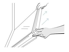
4. Remove the upper metal cover by pulling it upwards.
