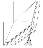
3. Remove the screws at each side of the door.
