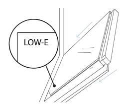
6. Once clean, carefully refit the glass and ensure the 'LOW-E' label is on the left side of the door, close to the hinge. The label will be inside the door.
