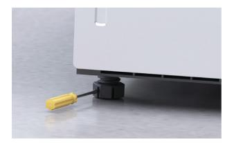
1. Using a flat bladed screwdriver, turn to raise the leveling feet. Level the rear, outside legs first followed by the front legs. Do not adjust the rear middle leg yet.
