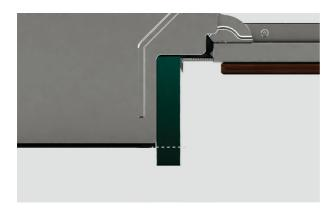
1. Align both sound seal sheets to the base of the dishwasher. If required, trim excess felt.
