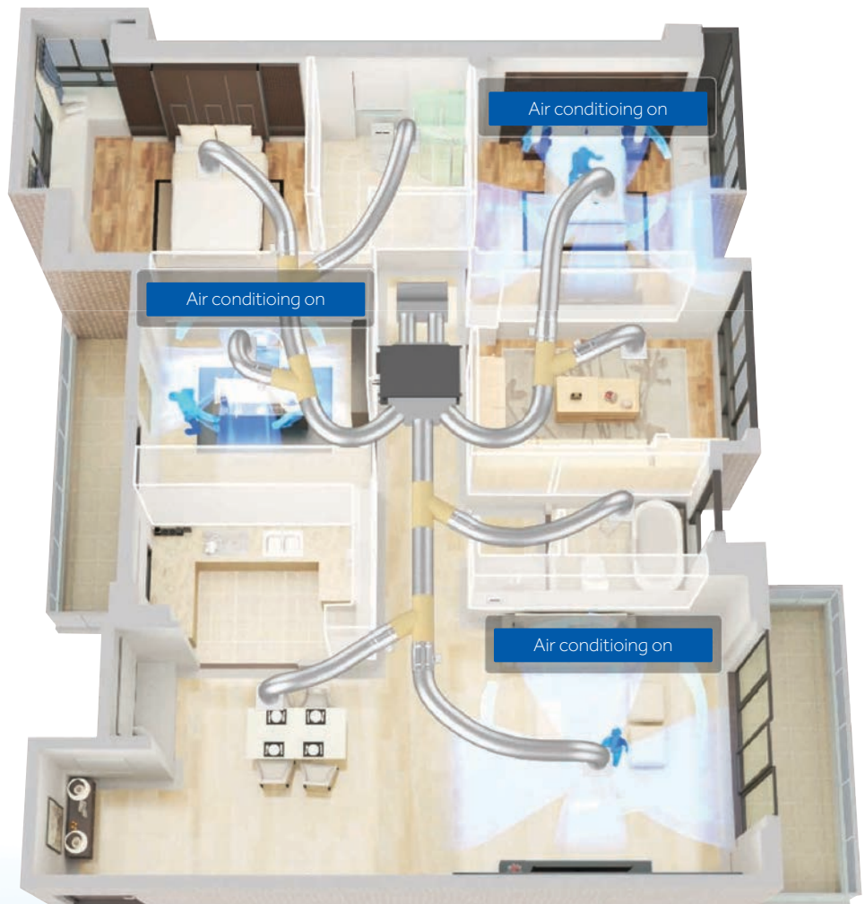
With SmartZone installed, air conditioning is switched on for only the three occupied rooms.
