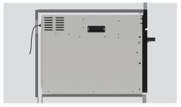
**4.** Ensure cavity ventilation has been set up correctly.
