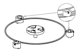
1. Position the turntable wheel guides correctly on the mechanism so that the rollers are at the top.
