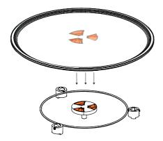
2. Place the glass turntable plate correctly onto the wheel guides.
